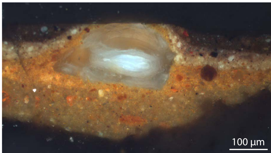
Fig. 1 Dark-field cross-polarized microscopy image of a large inclusion formed in the orange ground identified as lead soap in a paint cross-section from the painting Let the Children Come to Me by Jan de Bray (1663, Frans Halsmuseum). Picture by L. Abraham.
